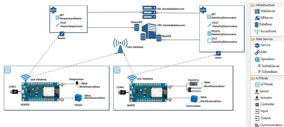
**Fig. 2.** Partial view of the graphic editor to model IoT scenarios.
